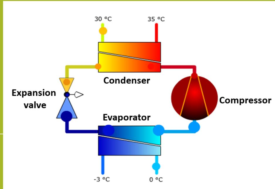
The refrigerant passes through an expansion valve where it drops its temperature and becomes a liquid once more, ready to continue the cycle.
